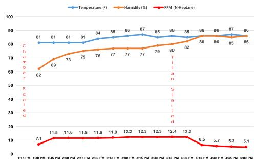
Chamber was sealed at 1:15 PM with a 100 cfm circulating fan running and 1 tbl spoon of N-Heptane in a beaker. Chamber was let set dormant for 2 1/2 hours to allow N-Heptane to fully evaporate and come to steady state. A Titan 1000 Hydroxyl Generator was turned on at 3:45 PM.
